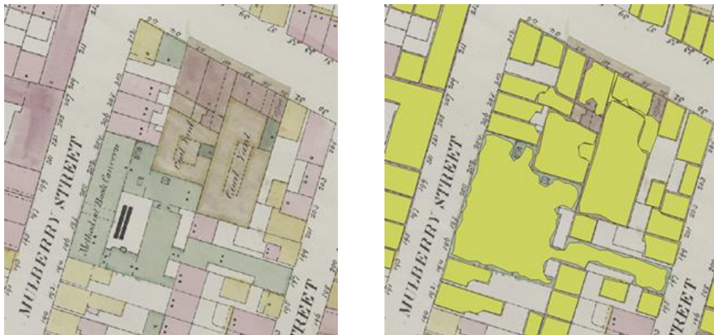
Figure 8: Example input and output from the map-vectorizer project. Images downloaded from https://github.com/nysl-spacetime/map-vectorizer , August 2019.
